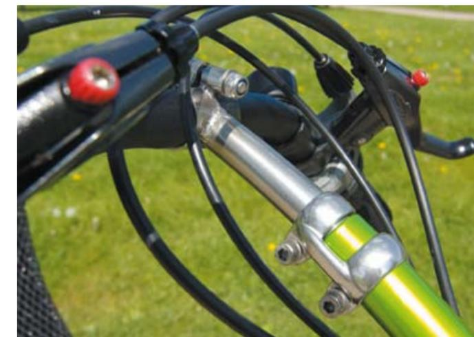
**ABOVE LEFT:** The stem folds on this stainless steel bracket, with a bolt to set its resting angle. Ours needed a touch of threadlock!
